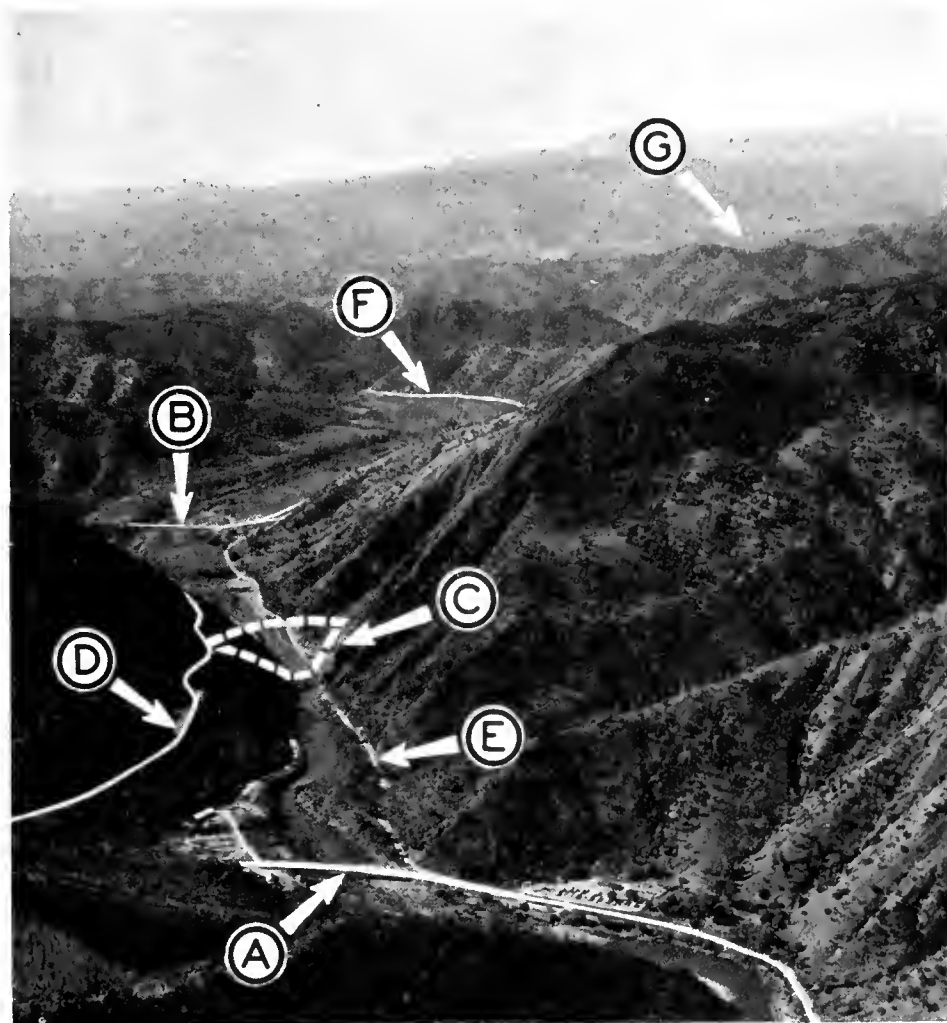
(A) Permanent bridge across Putah Creek; (B) Temporary bridge across Putah Creek; (C) "Devil's Gate" damsite, Monticello Dam; (D) Relocated highway, Unit No. 1; (E) Highway Route 6 now abandoned; (F) Highway Route 6 to be abandoned; (G) Berryessa Valley
